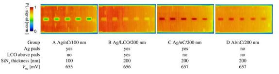
Fig. 2. Normalized PL-oc images of solar cells fabricated with different  $SiN_x$  layer thickness and combinations of LCOs and Ag pads. The images show the same close-up as in Fig. 1 and the pads are located between the front side busbars to avoid their shading during measurements. The open circuit values are averages of three cells each.
