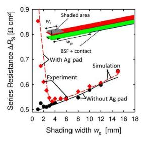
Fig. 4 Measured (symbols) and simulated (curves) series resistance  $R_s$  in dependence on the shading width  $w_s$  for cells without (black) and with Ag pads ( $w_p = 3.2$  mm, red). The inset shows a part of the unit cell indicating  $w_p$  and  $w_s$ .
