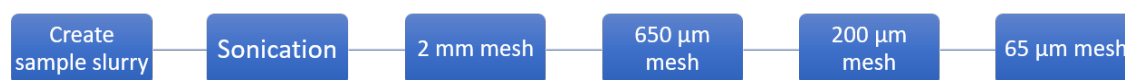
Fig. 3.2 The first step in sample preparation was fractionation for particle size. First, a slurry of sample material in Deionized Water (DI-water) was created to avoid whirling up dust. To break up potential particle agglomerates, the slurry was sonicated in an ultrasonic bath before filling the slurry into the first sieve. Here, four mesh sizes were used: 2000, 650, 200 and 65 \mu\text{m} . All sieves were stacked on top of each other, with a beaker underneath the bottom one to catch the resulting slurry with particle sizes <65 \mu\text{m} .
