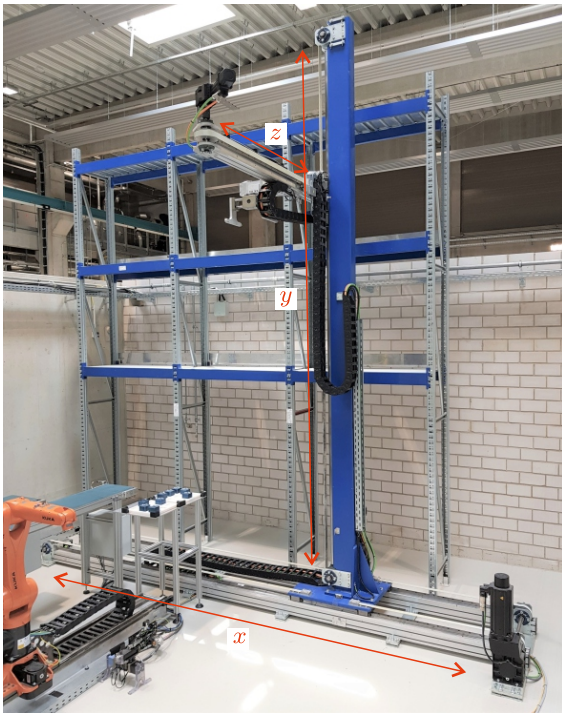
(b) Stacker crane
