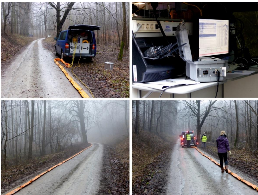
Figure 15: Shear-wave reflection seismic investigation at the Harz Boundary Fault.
