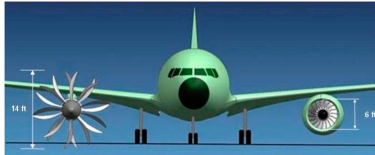
**Figure 5.** Large propeller installation issues for a low wing aircraft configuration.
