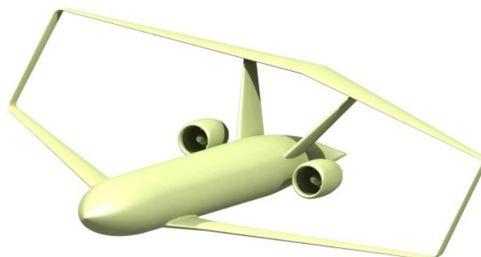
**Figure 9.** CAD model of the reference PrandtlPlane.
