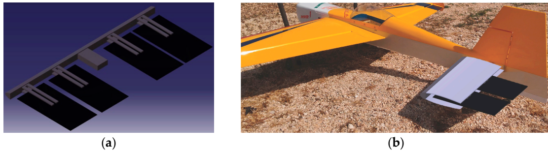
Figure 18. New horizontal tail concept: (a) bistable horizontal tail in CATIA and (b) UAV equipped with the concept of a horizontal bistable stabilizer.
