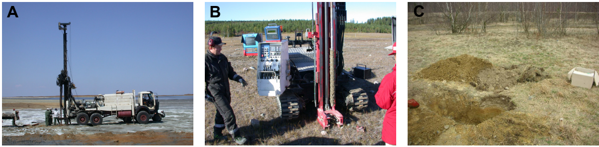
Fig. 2. In this thesis investigated mine waste tailings dumps. A: The drilling vehicle on top of the tailings dump located near Selebi-Phikwe in Botswana which was still in operation 2003 (see also Fig. 1). B: The drill rig on top of the remediated tailings dump near Kristineberg in Sweden. C: The outcrop on the unremediated tailings dump near Freiberg in Germany (Pictures A, B: Axel Schippers, BGR Hannover).
