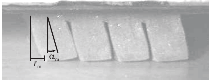
Figure 5.14: Deformation shape of siped tire tread block sliding on ice, captured with a high speed camera during a friction experiment with HiLiTe
