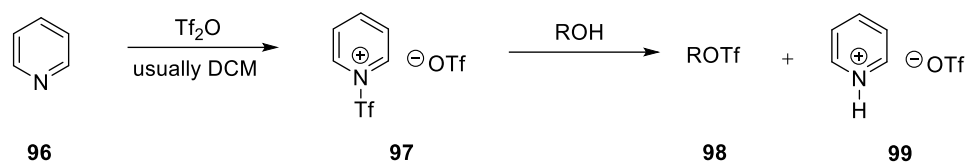
Scheme 2.17. Trifluoromethanesulfonylation of alcohols using trifluoromethanesulfonic anhydride and pyridine. [33]
