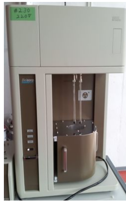
Figure 3.3.: Picture of the BELSorp max volumetric, static gas adsorption apparatus located in DIK Hannover.
