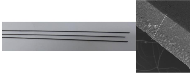
Figure 2: Light microscopic and scanning electron microscopic images of gas-tight LCCF capillaries
