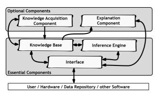
Fig. 1. Main Components of a Knowledge-Based System (acc. to [8])
