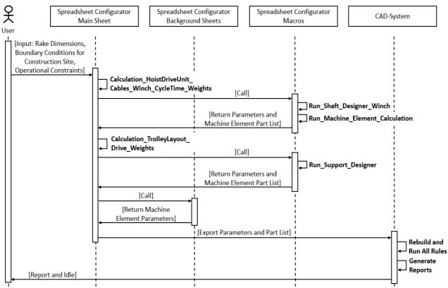
Fig. 8. Sequence Diagram for Trash Rack Cleaner Configuration
