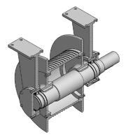
Fig. 5. Cable Drum (Sectional View)
