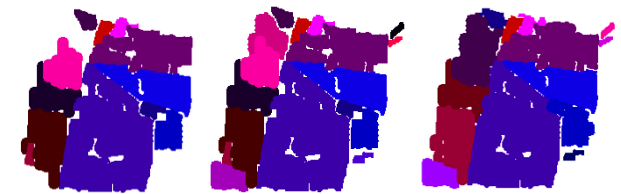
Figure 5. Left: results after adding new segments based on the point cloud to the results in Fig. 4. Centre: results after the second segmentation. Right: results after merging co-planar segments and filling small gaps.
