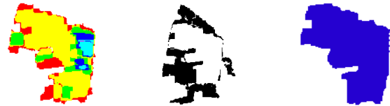
Figure 3. Left: overlap count for the best planar segment (segment B) in Fig. 1. Red / yellow / green / blue / cyan: 1 / 2 / 3 / 4 / 5 overlapping segments. Centre: regions belonging to non-co-planar matching candidates (black). Right: final roof segment.
