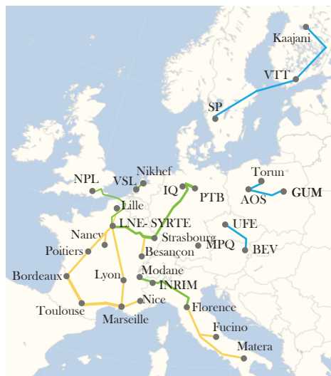
Figure 4.3: Optical fiber networks in Europe. Frequency links are shown in green, frequency links commissioned in yellow and time links in blue [64].
