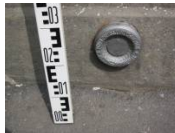
Figure 3.15: Picture of the reference Point of the LUH in respect to the geoid. Source: [58].
