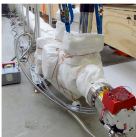
Figure 4.5: Bake-out of the baseline vacuum chamber.
