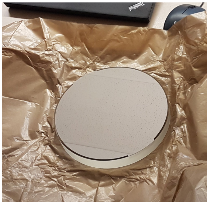
Figure 3.20: Picture of a new large mirror for future alignment. The mirror (fabricated by ‘Union Optics’) has the flatness of \lambda/4 and protected-silver coating on a substrate with 200 mm diameter.
