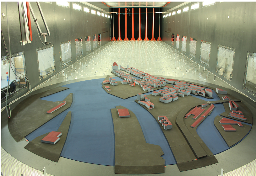
Figure 1. Photograph of the building setup within the wind-tunnel facility “WOTAN” for an approaching flow of 290^\circ . Please note that contrary to the depicted orientation, an approaching flow from 110^\circ was used in this study.
