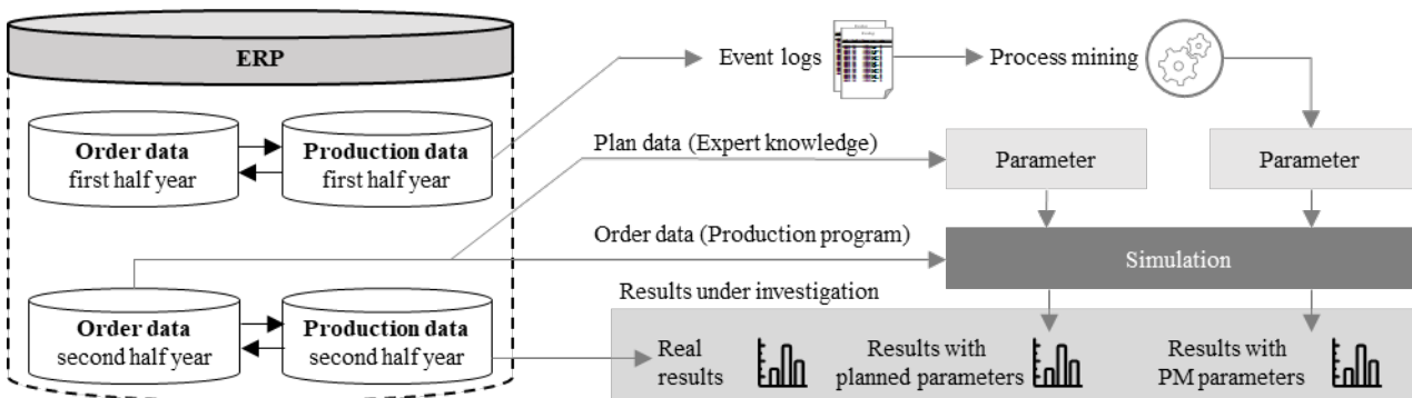
Figure 3: Comparison of real production data versus simulation scenarios by planned data and PM
