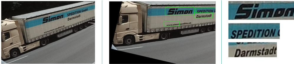
Figure 7: Example of text recognition on the vehicle body
