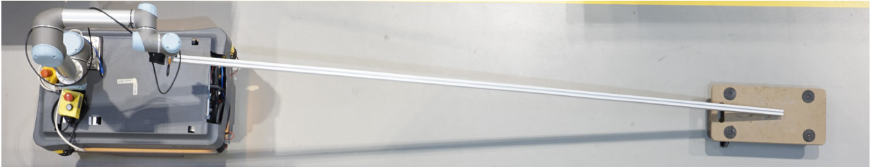
Figure 1: Top view of a mobile manipulator (MuR 205) transporting an aluminium construction profile in combination with a roller board
