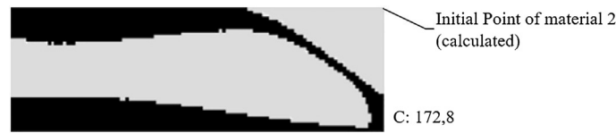
Fig. 5. Design of a MBB beam using IZEO (30 × 90 mesh; mass constraint of 50%; elasticity E_2 = 0.34 \times E_1 ; \epsilon_{r12} = 0.2\% in volume; S_a = 10\% in mass).
