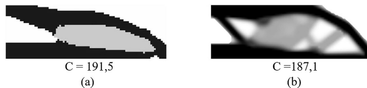
Fig. 8. Comparison between MBB design with IZEO and alternating active-phase algorithm. Both simulations present the same mesh, elasticity values, and volume fractions.
