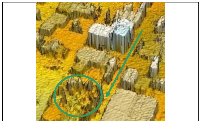
Figure 11: DSM by matching with SGM, green arrow = street
