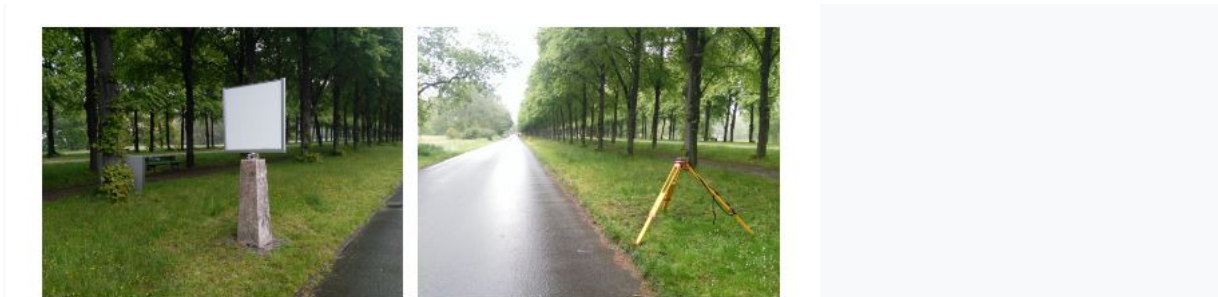
Fig 7: Outdoor experiment, Herrenhäuser Allee, Hannover, Germany. The panel is 43 % white. The ranges were varied between 75 and 200 m (Jüngerink 2019).
