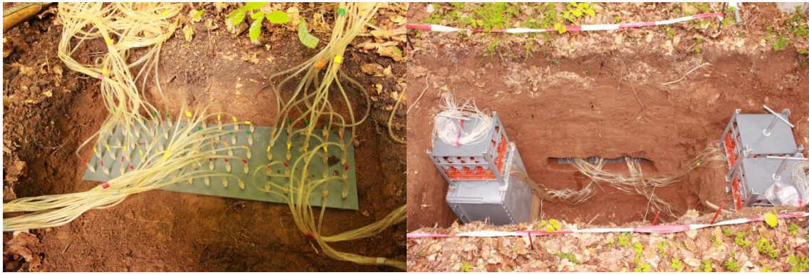
Fig. 1 Injection of DOC at 10 cm depth at the Red Sandstone site (left) and in 50 and 100 cm depth at the Loess site (right). Note that on the right site, the injection at 100 cm depth is shown. The injection at 50 cm depth was conducted on the opposite site. The injection area was designed for three possible samplings.
