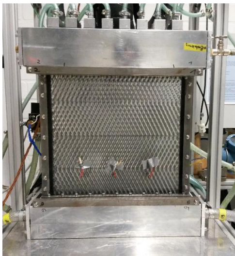
Figure 3. Transparent corrugated adiabatic test section (corrugation angle of 27°)
