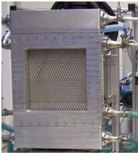
Figure 5. Test section for the diabatic experimental setup (corrugation angle of 27°)
