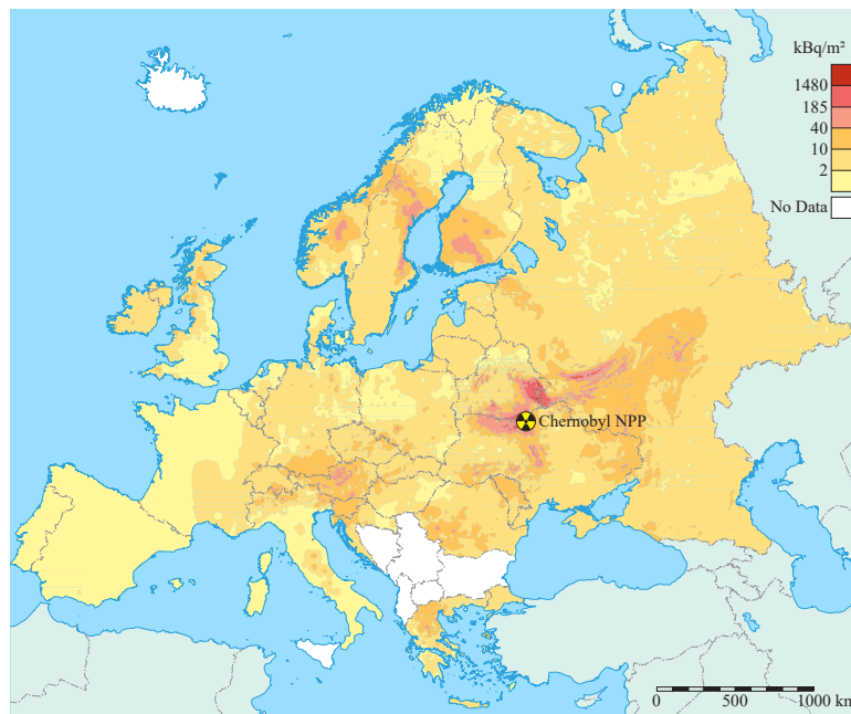
Figure 1.11: Surface contamination in \text{kBq/m}^2 for ^{137}\text{Cs} of Europe due to the Chernobyl accident in 1986. Adapted from UNSCEAR. 63
