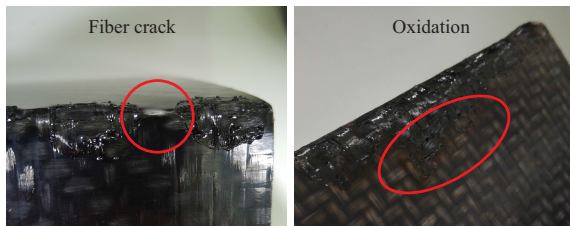
Fig. 11. Fiber failures (left: fiber cracks, right: matrix oxidation)
