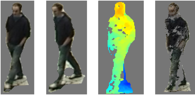
Figure 3: Input to dense matching (left), colour-coded disparity map (center) and coloured point cloud (right).
