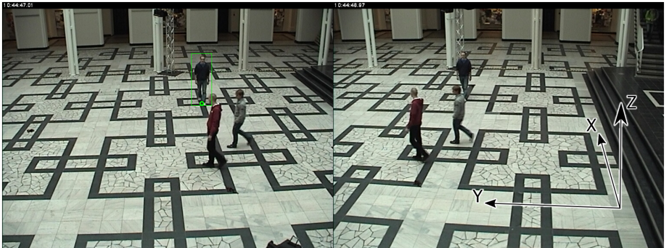
Figure 5: Stereo image pair from test sequence. The coordinate system is translated into the image to show the directions of the axes. In the left image a bounding box is depicted as well as the position derived from our approach (green circle).
