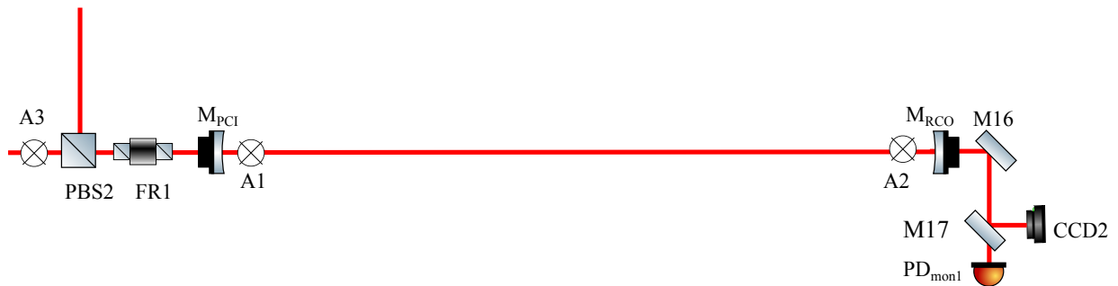
Figure 4.14: Second step of the alignment procedure for the overlap performance: the curved mirrors are aligned to the optical axis by adjusting their reflections to the apertures A1, A2, and A3. For simplicity, the HPL and its corresponding components are not shown.
