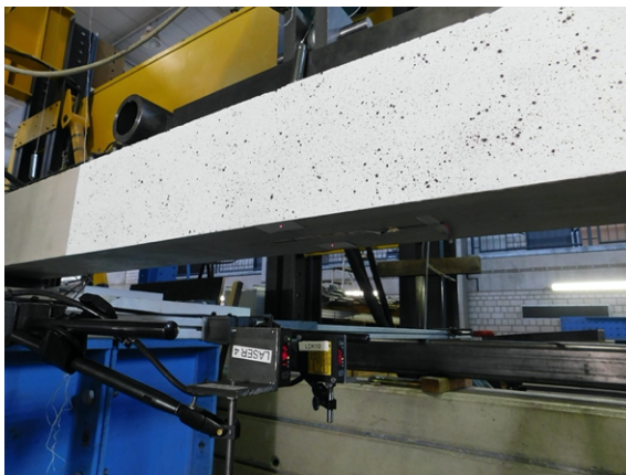
Figure 8.3: Laser distance sensors for measuring the deflection of the beam in the middle
