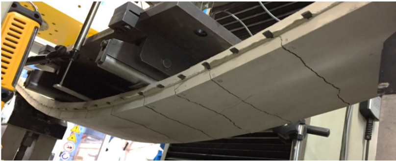
Figure 8.11: Four-point bending test of a mid-scale slab with carbon textile reinforcement
