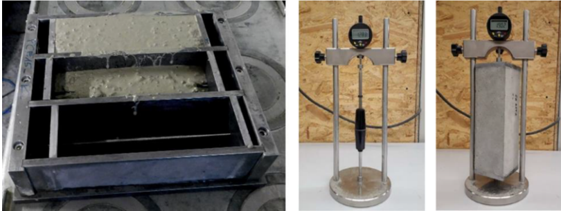
Figure 6.1: Restrained Expansion Test: concreting the specimens and measurements of the comparator bar and of the specimen
