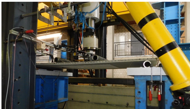
Figure 8.17: Test setup for four-point bending of a concrete slab with carbon textile reinforcement
