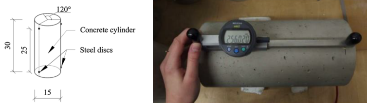
Figure 6.2: DEMEC strain measurements: schema and specimen during measurements
