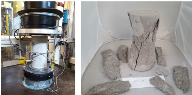
Figure 5.1: Compressive test of a concrete specimen and a picture after failure
