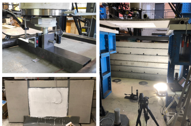
Figure 8.18: Laser distance sensors for measuring the deflection of the slab in the middle (left top), preparation of the DIC area (left bottom) and DIC setup for capturing the crack pattern (right)
