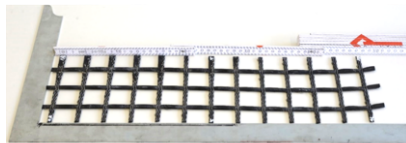
Figure 4.1: Textile reinforcement solidian GRID Q142/142-CCE-38
