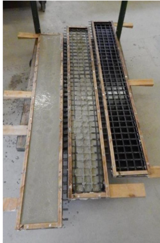
Figure 4.8: Mid-scale slab specimens during concreting
