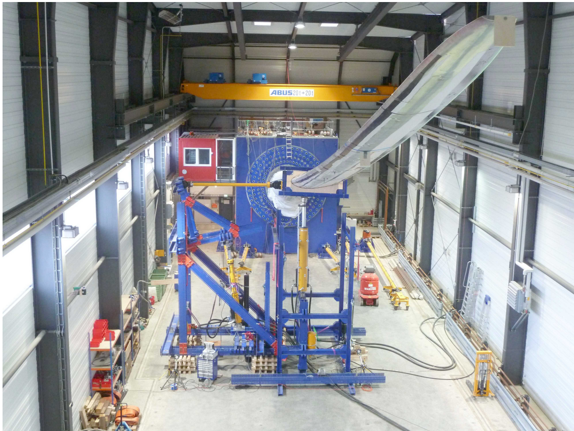
Figure 4.1: Test setup of the biaxial dynamic fatigue test. View from the blade tip.
