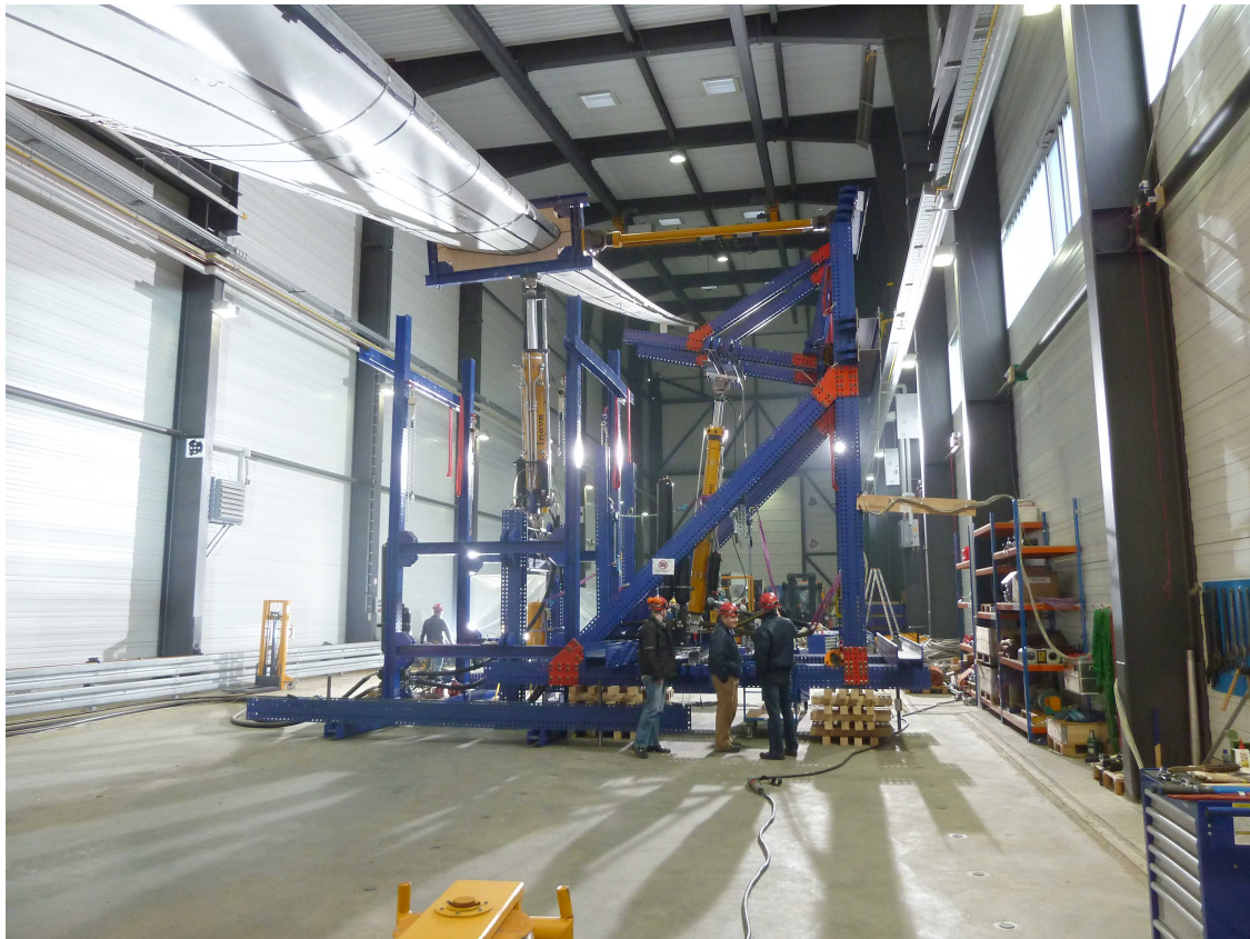
Figure 4.2: Test setup of the biaxial dynamic fatigue test. View from the blade root.
