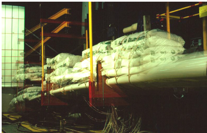
Figure 1.3: Fatigue test in flap-wise direction of the DEBRA-25 blade, carried out in 1983/84. Four load frames and a whiffletree structure were used in combination with a hydraulic actuator to lift the blade up. Sandbags were used to apply the specified loading when unloading the actuator. 40,000 cycles were applied at different amplitudes.
