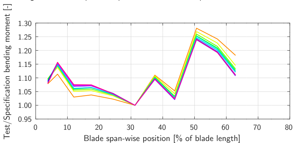
Figure 4.7: To be comparable, all curves of Figure 4.6 were scaled linearly to be 1 at 31% of the blade length. The deviations of up to 6% at 60% to 70% of the blade length are likely caused by aerodynamic drag forces.
