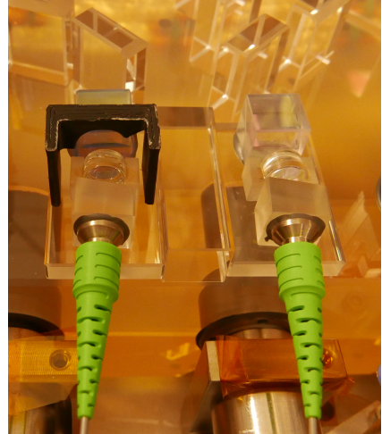
Figure 12.6.: Polarisation filter on the spare OB filter before PBS .
