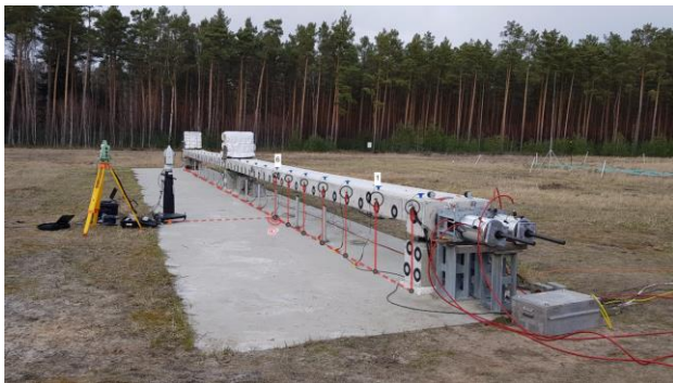
Figure 5. The BAM synthetic bridge measured by the MEMS accelerometers, the laser tracker and the IATS.
