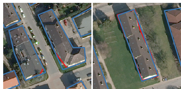
Figure 5. Regularization of building footprints by completing corners (left) and improving parallelism of opposite edges (right). Input vector in red and regularized vector in blue.
