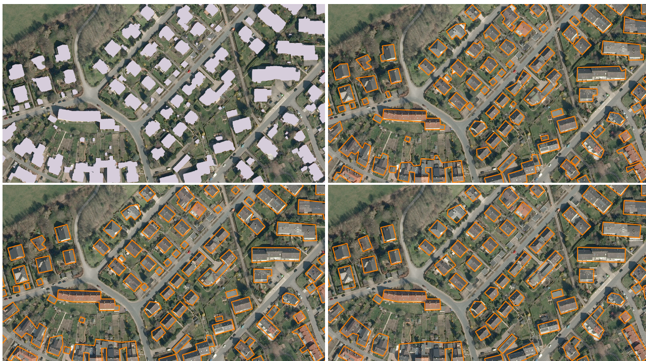
Figure 6. Building blobs from land cover classification (upper left) and generated building vectors at map scale 1:10,000 (upper right), 1:15,000 (lower left), and 1:25,000 (lower right)
