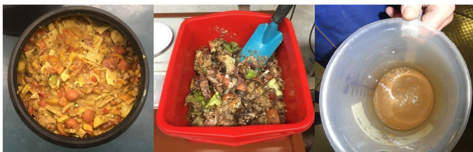
Fig. 2 Substrates onboard cruise ships: (left) food waste; (centre) dewatered food waste; (right) sewage sludge
