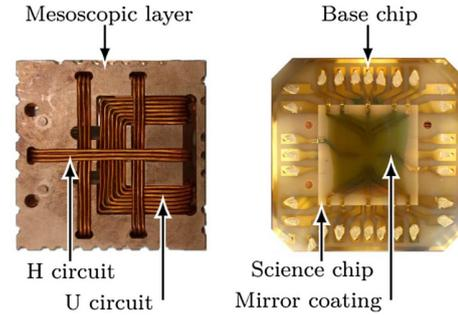
**Fig. 3.** Photograph of the atom chip assembly. The mesoscopic layer produces magnetic fields for the MOT configuration and the transfer to the Ioffe–Pritchard-type trap provided by the chips. The Base and Science chip provide the magnetic fields for transfer and the final trap geometry for efficient evaporation. The mirror coating is used for the MOT configuration and redirects the interferometry beam.
