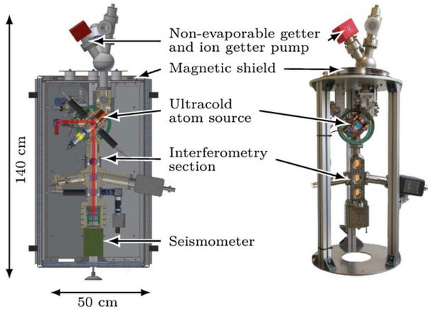
**Fig. 1.** Photograph and conceptual design section view of the sensor head of the QG-1 setup. The photograph depicts the system before mounting of the collimation and detection optics, as well as the magnetic shield. In the section view the interferometry laser beam path is highlighted.
