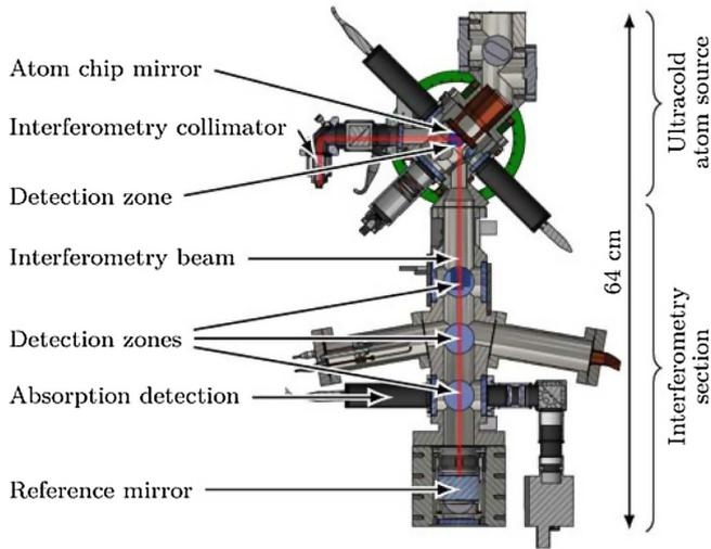
**Fig. 4.** Conceptual design section view of the high-flux source and the interferometry section. The collimated and polarisation purified laser beam enters the experiment chamber through a vacuum window, is reflected at the atom chip mirror and retro-reflected by a tilt-able mirror of high optical quality. The atomic sample can be detected by absorption imaging at four detection zones.
