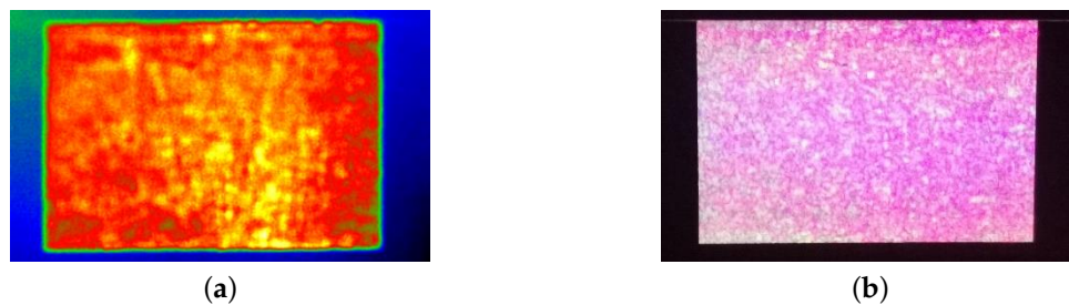
Figure 8. Projection and measuring results of the investigation setup. (a) The measured luminance image from the LMK Color 5; (b) The real projection photo.
