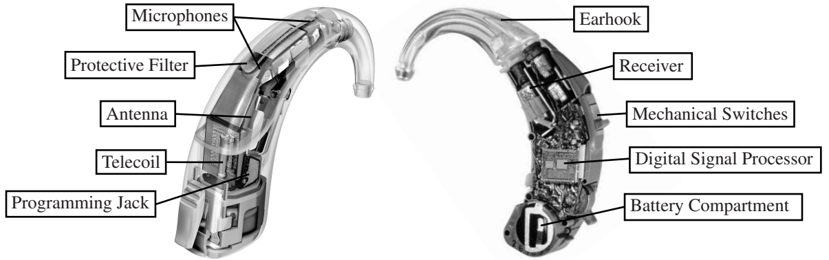
Figure 2.1: Schematic view and photograph of a behind-the-ear (BTE) hearing aid [17, 18].
