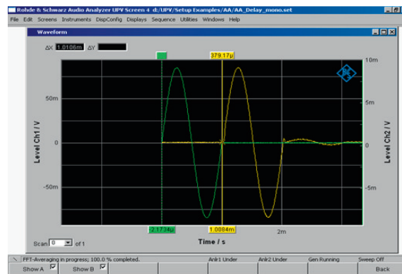
Figure 3.73: Measurement of the analog-to-analog audio latencies of audio processing systems. A audio analyzer connected to the analog in- and outputs of the external audio codec. The first sine wave is generated by the audio analyzer and is used as an input for the audio codec. The second sine wave is measured at the output of the audio codec. The latency is the time delay between these waves.
