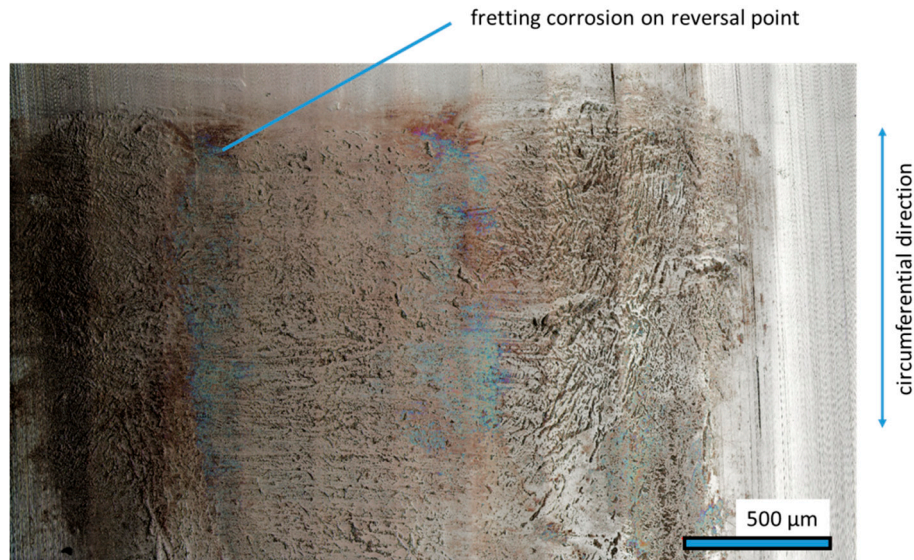
Figure 8. Raceway surface on reversal point for grease-lubricated bearing after more than 1 million oscillating cycles, the formation of tribofilm and fretting corrosion.
