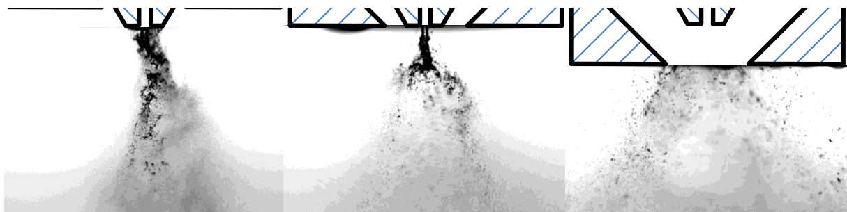
(c) Condition 3: Q_a / Q_w = 3800 (Nozzle cover position 1 to 3 from left to right)
