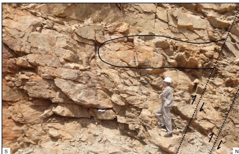
Figure 12. Pegmatite body emplaced in horizontal extension fracture (black line) associate with reverse fault plane (dotted black lines).
