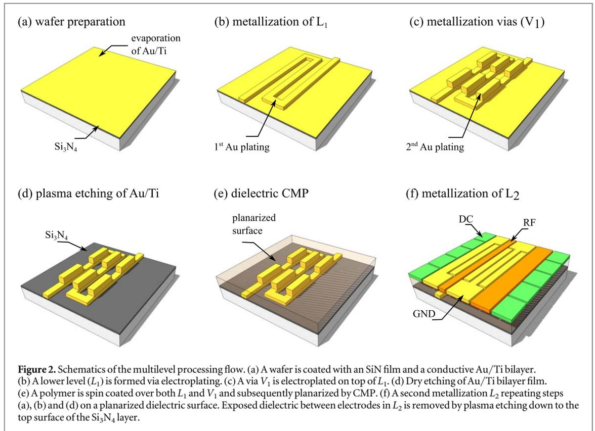
Finally, after gold electroplating the resist mask is removed chemically and the wafer is cleaned under oxygen-based plasma etching. Additionally, the wafer is exposed to a fluorine-based plasma to further remove possible resist debris. Immediately afterwards the seed Au layer is removed via Ar etching and the Ti layer removed by a fluorine-based plasma etching.
