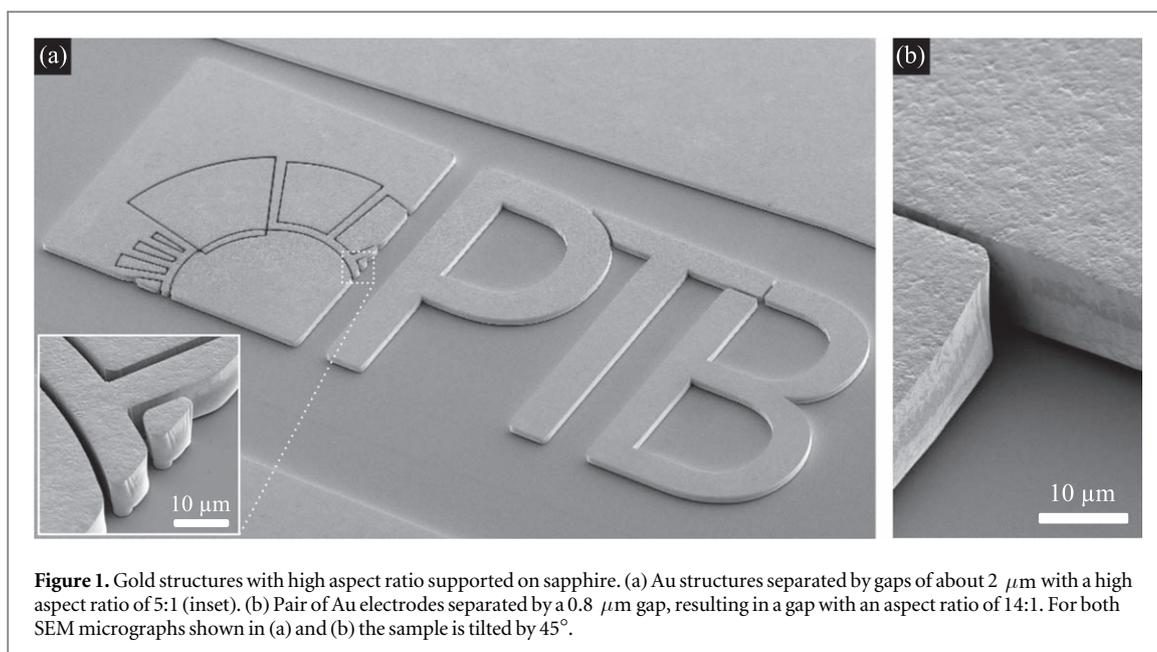
**Figure 1.** Gold structures with high aspect ratio supported on sapphire. (a) Au structures separated by gaps of about  $2\ \mu\text{m}$  with a high aspect ratio of 5:1 (inset). (b) Pair of Au electrodes separated by a  $0.8\ \mu\text{m}$  gap, resulting in a gap with an aspect ratio of 14:1. For both SEM micrographs shown in (a) and (b) the sample is tilted by  $45^\circ$ .
