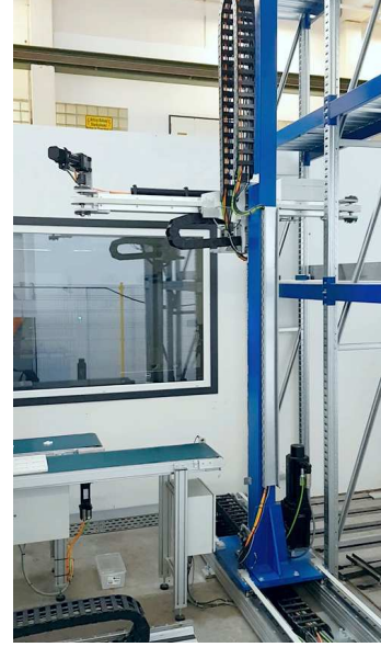
Fig. 2. Experimental testbed: stacker crane
