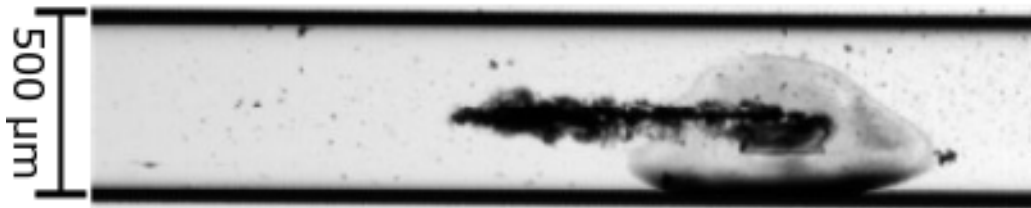
Fig. 5: Damage morphology observed in a PMMA fiber under exposure to laser radiation at 532nm and a pulse duration of 7.3ns [59].
