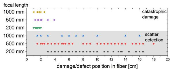
Figure 4. Positions of scattering centers and catastrophic damage along the fiber for three different focal lengths of the focusing lens. The fiber mount prevents a detection of scattered light within the last 1-2 cm thus the data is not shown here.
