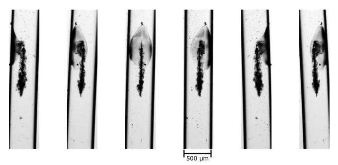
Figure 8. SLOT images of one fiber and the laser-induced damage for catastrophic damage close to the fiber core center at different angles. Light propagated from bottom to top.
