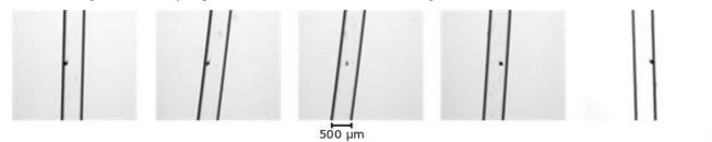
Figure 6. SLOT images of one fiber and the laser-induced damage for LLSC and MTL at different angles. Light propagated from bottom to top.
