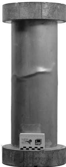
Figure 3. UHPC hybrid tube specimen after testing the axial load carrying capacity. A buckling figure can be seen on the outer surface of the outer steel sheet. In this area the concrete core is locally destroyed. However, due to the lateral supporting effect of the steel sheets, normal forces can still be absorbed. The residual load is made up of different components. On the one hand, sheet steel reinforcement can absorb further normal forces and on the other hand, the broken concrete core can also transmit normal forces due to the lateral supporting effect of the sheet steel.[2]
