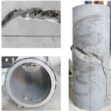
Figure 2. Test specimen (pure UHPC hollow section with steel fiber reinforcement) after testing the axial load carrying capacity. After reaching the maximum load-bearing capacity, no further loads could be applied. The residual load bearing capacity tends towards zero.
