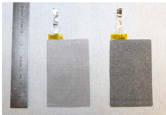
Figure 1. LTO reference electrode. Uncoated aluminum mesh (left) with current collector tap already welded on. Aluminum mesh after dip coating with LTO (right).
