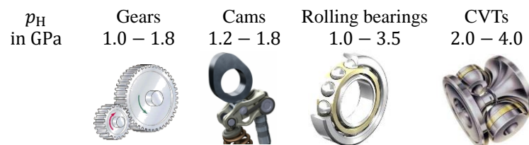
Figure 1-4: Contact pressure in some rolling/sliding EHL lubricated transmission components [the pressure values refer to Zhang, Spikes 2020]
