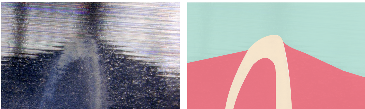
Figure 2.34: Pitch bearing raceway with wear damage modes
