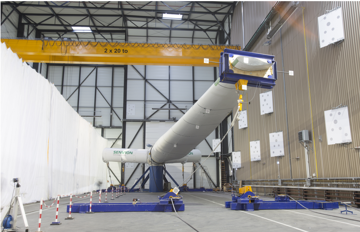
Figure 2.42: Fraunhofer IWES initial pitch bearing test rig for Senvion ©: Fraunhofer IWES / Martina Buchholz
