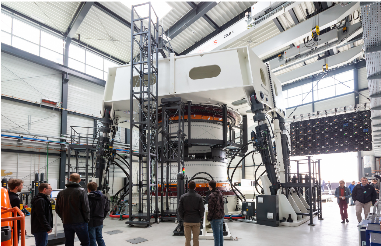
Figure 5.5: BEAT6.1 test rig with hybrid Force Transmitting Element ©: Fraunhofer IWES / Ulrich Perrey
