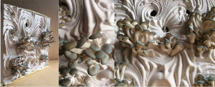
Figure 4. Facade element fabricated at IAAC using digital manufacturing optimized to grow Oyster Mushroom
