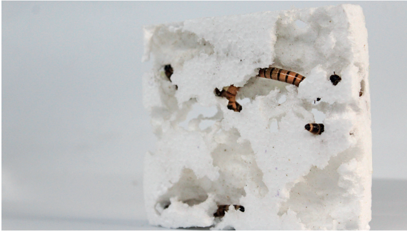
Figure 1. mealworms within porous eaten polystyrene block © Eve Nnaji, Madhavi Ohja (2020)
